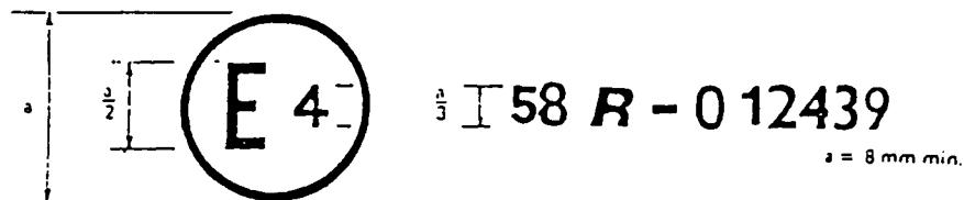
The above approval mark affixed to a vehicle or to an RUPD shows that the vehicle type or RUPD type concerned has, with regard to the rear underrun protection in the event of a collision, been approved in the Netherlands (E 4) pursuant to Regulation No. 58 under approval number 012439. The first two digits of the approval number indicate that the approval was granted in accordance with the requirements of Regulation No. 58 as amended by the 01 series of amendments.
