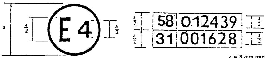
The above approval mark affixed to a vehicle shows that the vehicle type concerned has been approved in the Netherlands (E 4) pursuant to Regulations Nos. 58 and 31. 1/ The approval numbers indicate that, at the dates when the respective approvals were given, Regulation No. 58 included the 01 series of amendments and Regulation No. 31 was still in its original form.
